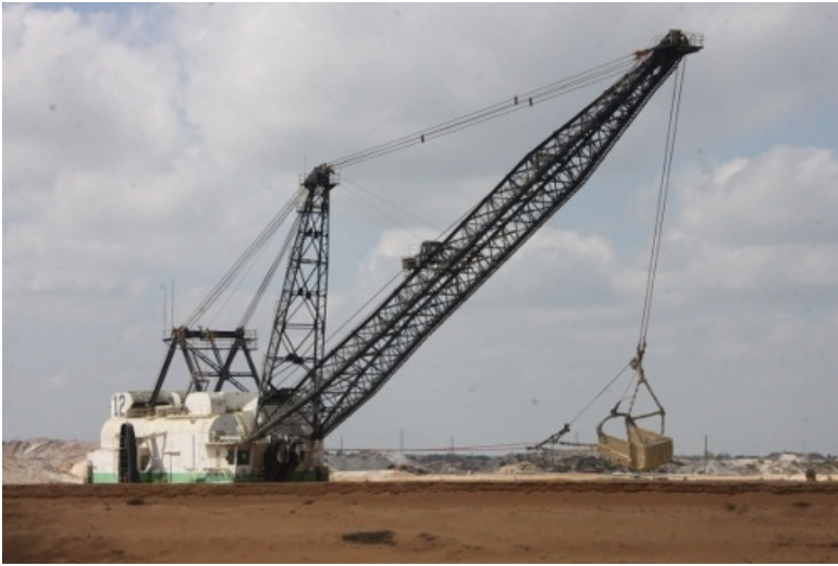
A “Walking Dragline” at work. The power unit is the height of a two-storey house, the jib is about 50 feet high, and the scoop could easily hold a couple of cars.
